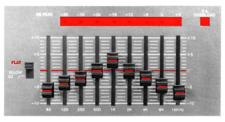
The graphic equalizer can also be used to produce disco-type sound by moderate amounts of low- and high-frequency boost.
